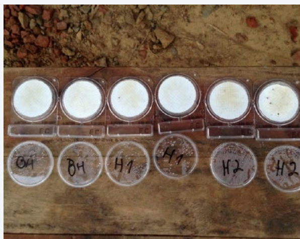
Figure 33: Using two handheld water quality probes to take manual measurements in Cox's Bazar, Bangladesh (left). A field testing kit for E.Coli and coliform bacteria used by Groundwater Relief in Cox's Bazar, Bangladesh (right). (GWR)
