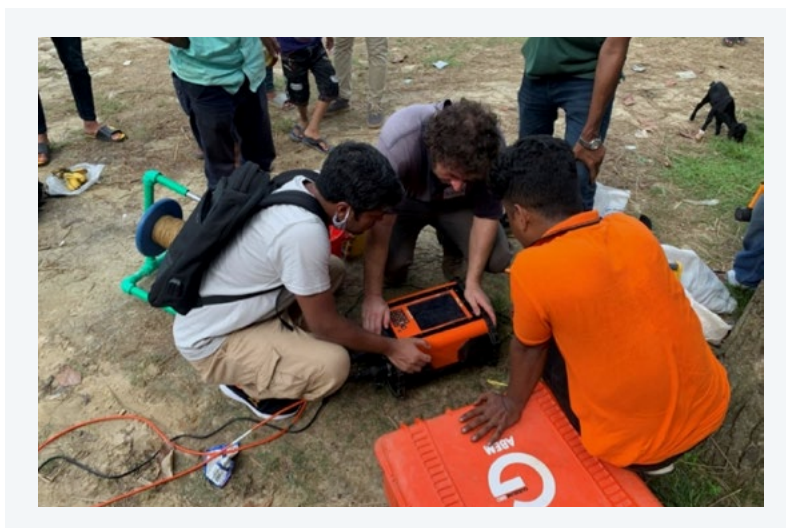
Figure 34: Groundwater relief supporting local technicians in setting up an electrical resistivity tomography (ERT) survey in Cox's Bazar, Bangladesh. (GWR)
