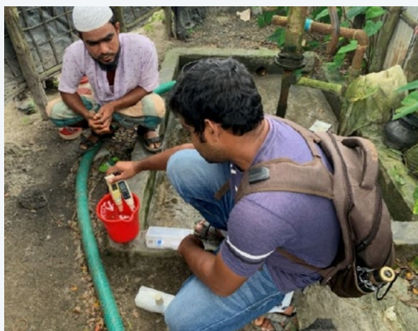
Figure 33: Using two handheld water quality probes to take manual measurements in Cox's Bazar, Bangladesh (left). A field testing kit for E.Coli and coliform bacteria used by Groundwater Relief in Cox's Bazar, Bangladesh (right). (GWR)
