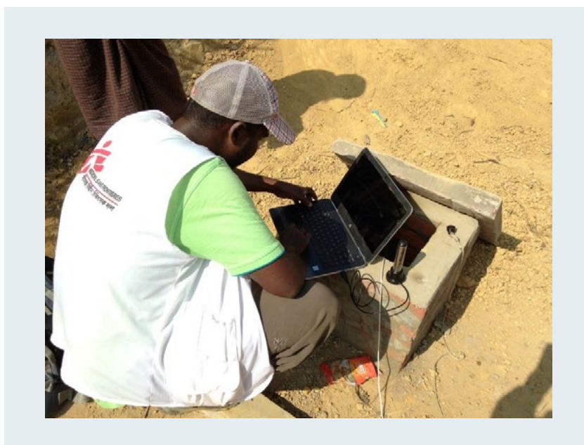
Figure A4: Technician setting up an In-Situ datalogger in Cox's Bazar, Bangladesh. (GWR) ( Water Monitoring Equipment, Water Quality Testing, & More | In-Situ 39 )
