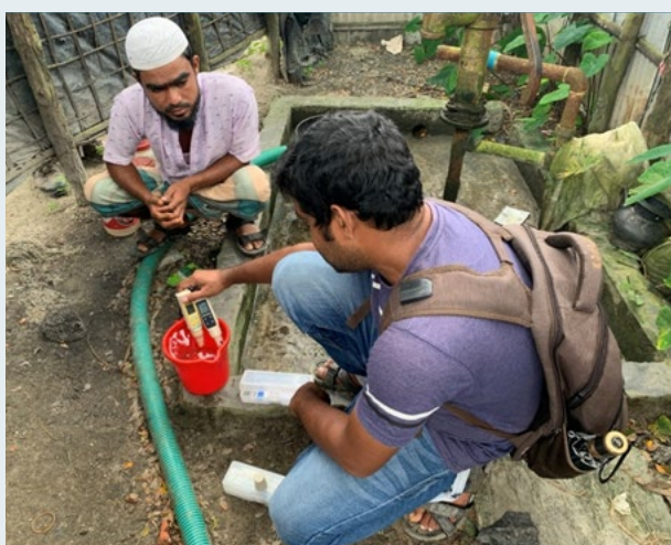
Figure A8: Using two handheld water quality probes to take manual measurements in Cox's Bazar, Bangladesh. (GWR)
